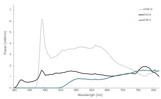
Visible power density curve of the short wavelength-optimized and low power lasers.
