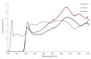
Visible power density curve of the high power lasers.
