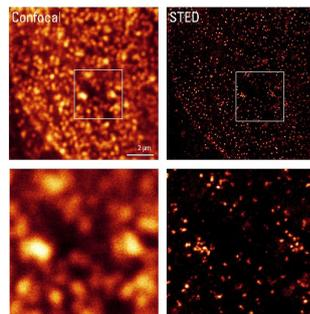
Resolution enhancement achieved with Leica TCS SP8 STED 3X microscope and the 775 nm Katana-08 HP pulsed laser, compared to the resolution achieved with confocal microscopy. Courtesy of Leica Microsystems
